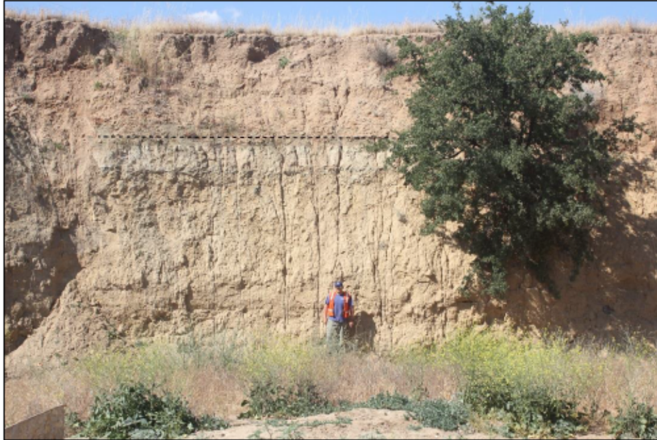
Photo 5. North-facing cut bank in Dry Creek showing the subsurface geology of an area less than 1 kilometer northeast of the Creston Route at Survey Point I. For scale, the individual shown is 6'2" tall. Dashed line represents the approximate boundary between the overlying alluvial sediments and the underlying Paso Robles formation.
